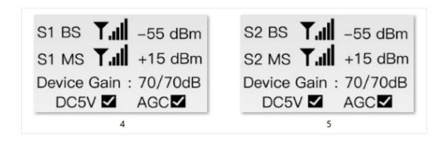
**LINE 1.** BS shows the level of outdoor incoming signal for the corresponding frequency band. Make sure it is as low as possible.
